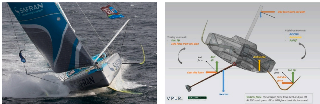
Fig. 18. Safran IMOCA 60 equipped with a canting keel and passive hydrofoil (IMOCA Globe Series, 2016; Stability and foils on the new IMOCA, the operating principles, 2017).
