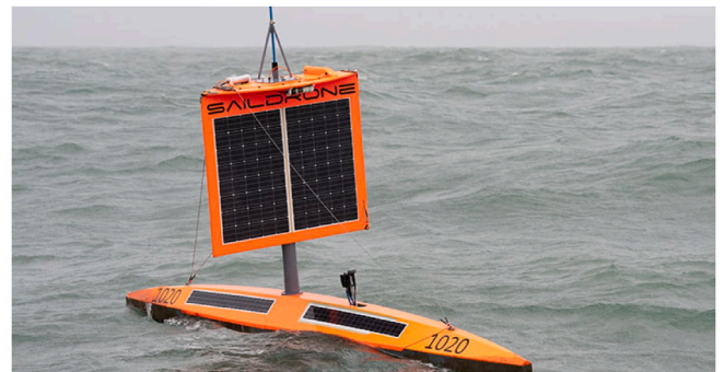
Fig. 14. Saildrone with a customized stubby sail (Clemens, 2019; Stein, 2019). Given the conditions in Antarctica, the Saildrone inevitably prioritizes overturning resistance to ensure survivability by adopting a stubby sail rather than the iconic slender sail.
