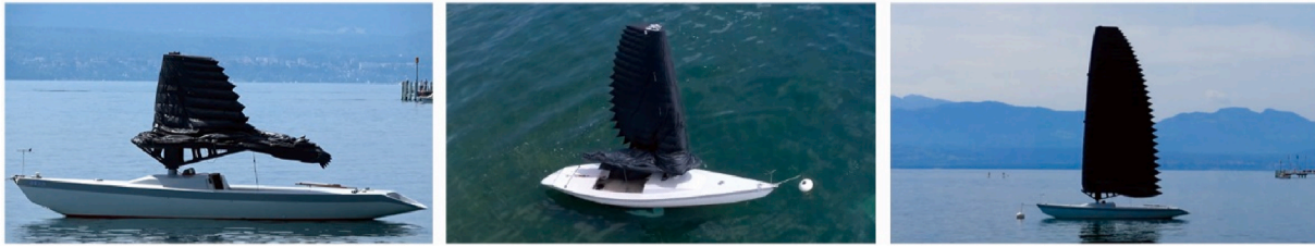
Fig. 16. Inflatable wing (Inflated Wing Sails, 2018). When the sail area of the inflatable sail requires modification, sail units deflate, the mast is lowered, and the deflated sail is placed in the nest.
