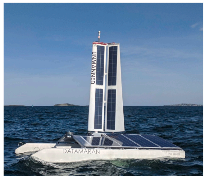
Fig. 3. Solar panels on the Datamaran Mark8 (PLATFORM — Autonomous Marine Systems, 2019). To enhance energy harvesting, Datamaran Mark8 makes full use of its large deck area to arrange solar panels.
