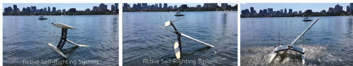
Fig. 10. Active self-righting system of the Datamaran ( PLATFORM — Autonomous Marine Systems, 2019 ). The active self-righting system allows the Datamaran to take full advantage of the good stability of the catamaran and overcome the shortcomings of being unable to upright itself after capsizing.
